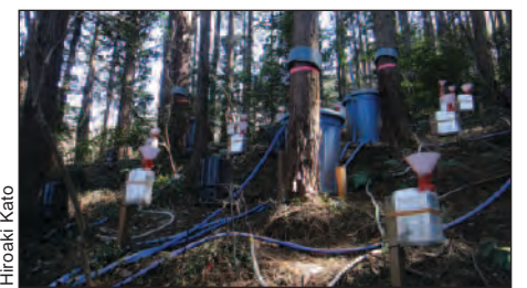
Researchers tracked the flow of radioactive particles by collecting water in cedar and cypress forests, as shown above.
